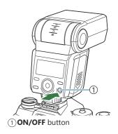
• When the flash is not in use, press the **ON/OFF** button to turn it off.
