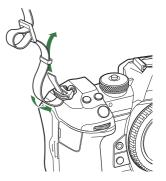
**3.** Pass the end of the strap through the buckle and tighten as shown.
