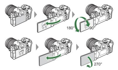
• Gently rotate the monitor within its range of motion. Attempting to rotate the monitor beyond the limits shown below could damage the connectors.
