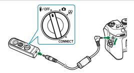
Rotate the mode dial of the remote control to **\fi/OFF** and connect the remote control to the camera via the supplied cable.
