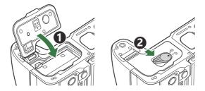
② Be sure the battery compartment cover is closed before using the camera.
