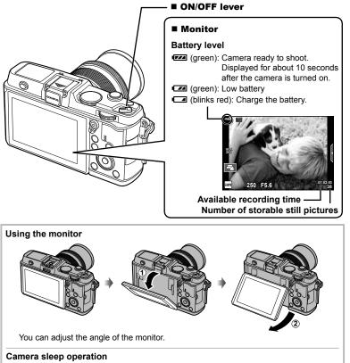
If no operations are performed for a minute, the camera enters "sleep" (stand-by) mode to turn off the monitor and to cancel all actions. The camera activates again when you touch any button (the shutter button, **>** button, etc.). The camera will turn off automatically if left in sleep mode for 4 hours. Turn the camera on again before use.
